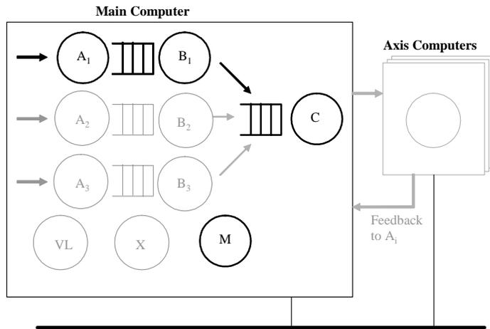
Figure 24: Tasks in the Robotics Model Problem
