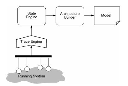
Figure 1: The DiscoTect Architecture
