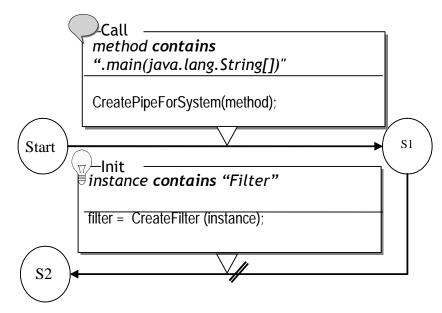
Figure 3: State Machine for Discovering Filter Components
