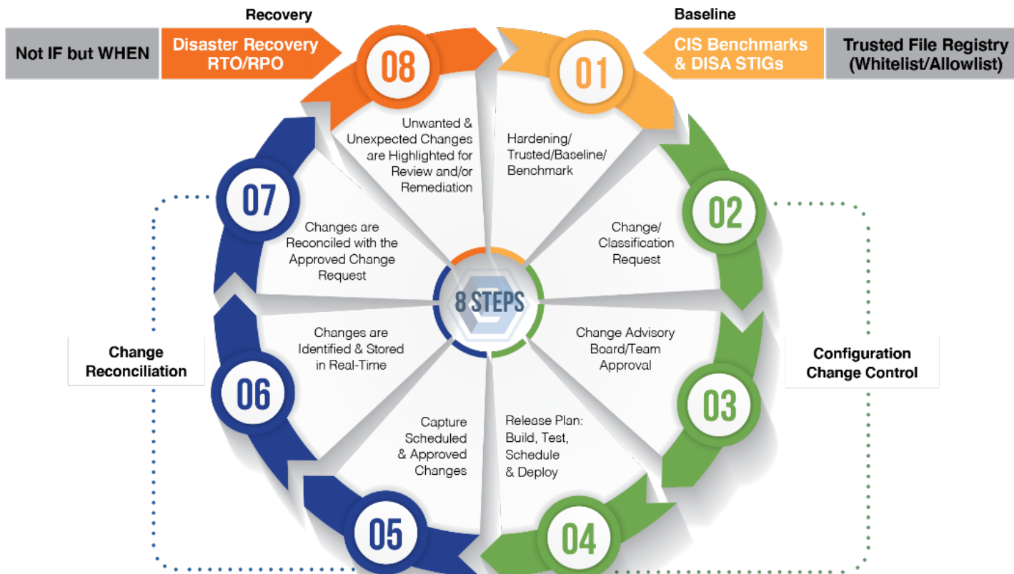
Model showing closed-loop change integrity assurance process. Image copyright of Cimcor Inc.
