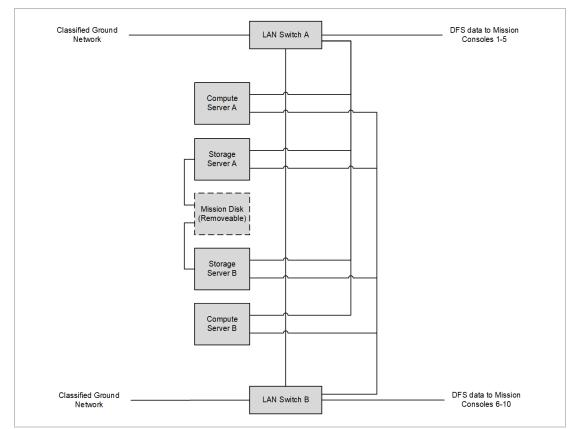
Figure 5: DSF Network Architecture
