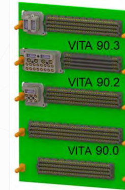
Example of VITA 90 VNX+ backplane and module
