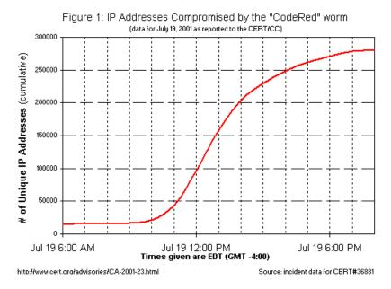
NOTE: After 8:00 PM EDT on July 19 (0:00 GMT July 20), the worm switched into flood mode on most infected systems, so the number of infected systems remained fairly constant after that time.
