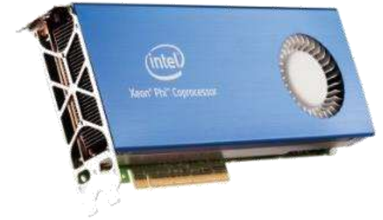
Intel Xeon Phi 7290F 1.7 Tflop/s, 260 W 72 cores, 1.5 GHz 8-way/16-way LRBni
