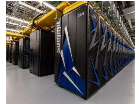
Summit 187.7 Pflop/s, 13 MW 9,216 x 22 cores POWER9 + 27,648 V100 GPUs
