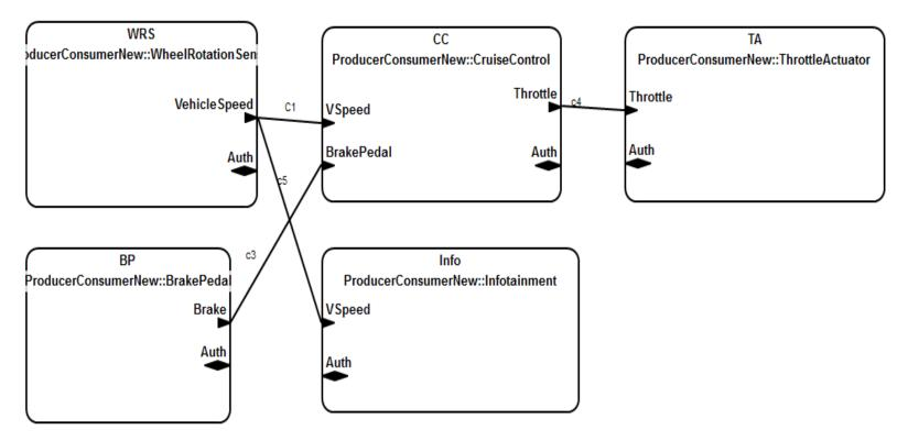
A subset of automotive electronics includes sensors (WheelRotation, BrakePedal), actuators (ThrottleActuator), and control application software (Cruise Control and Infotainment).
