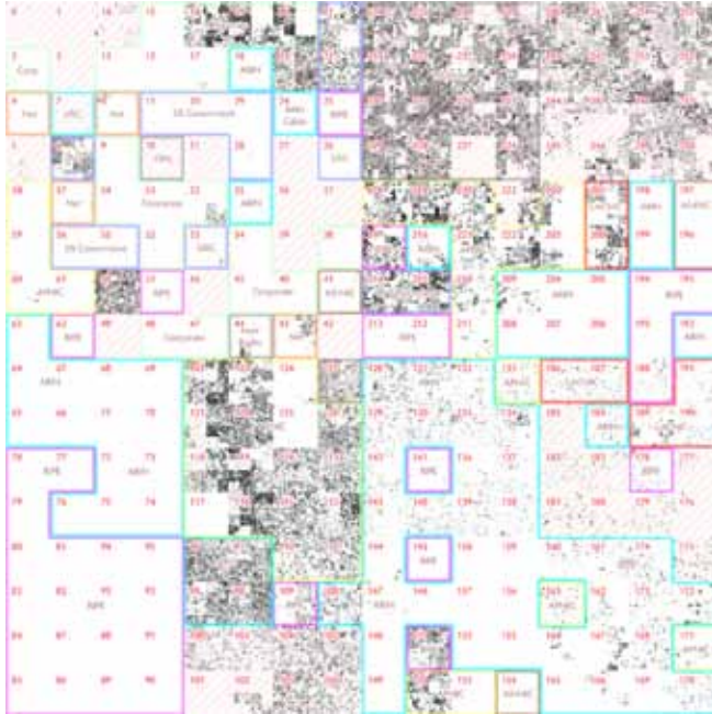
Figure 2: A visualization of network traffic generated using ryhilbert, a Rayon-enabled visualization tool that displays blocks of network addresses such that contiguous addresses are adjacent. Each point is a network block; blocks are shaded to indicate traffic volume, and colored borders are laid over the visualization to indicate IP allocations. Larger squares indicate larger networks; the red numbers in the “upper left” of blocks representing Class A networks show the first octet of those networks’ addresses.
