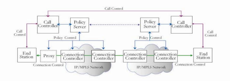
Figure 1. Reference QoS Control Architecture
