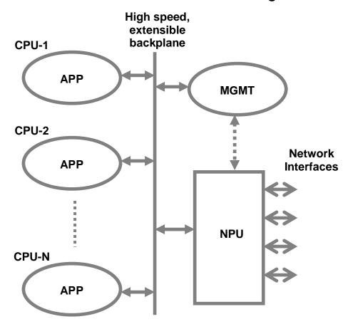
This architecture utilizes a combination of general purpose processors (CPUs) running the Linux operating system, and a new generation Network Processing Unit (NPU) for performing various flow operations. One processor (MGMT), also running Linux, is reserved for purely management functions, while other CPUs run applications. All of the
