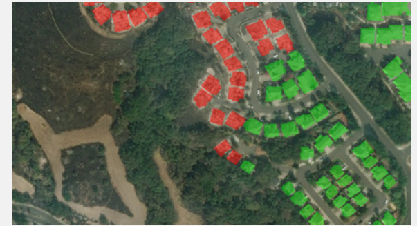
The xView 2 Challenge applies ML to help first responders detect and classify damage to structures.
