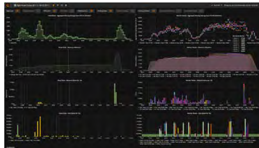
PMW's dashboard display using Grafana integrates with Elastic Stack to achieve complex visualizations. This example shows system metrics for a Spark MLlib job that uses one "head" node (displayed on the left) and eight worker nodes to perform a logistic regression algorithm (displayed on the right).
