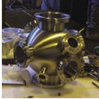
A custom, spherical high-vacuum chamber from the Kurt J. Lesker Company
