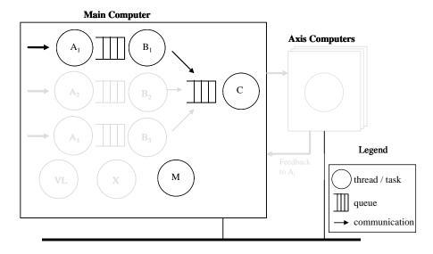
Figure 2: Tasks on the Main Computer
