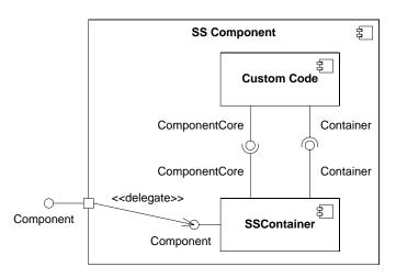
Figure 10: Using the Same Custom Code with a Different Container
