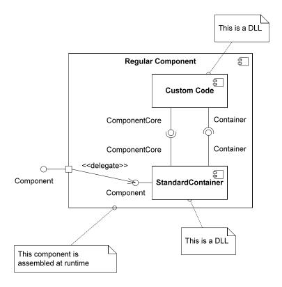
Figure 9: Component with the Container Idiom
