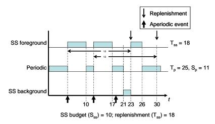
Figure 3: Example of a Sporadic-Server-Controlled Task
