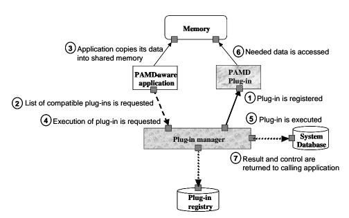
Figure 2: Component Interaction Diagram
