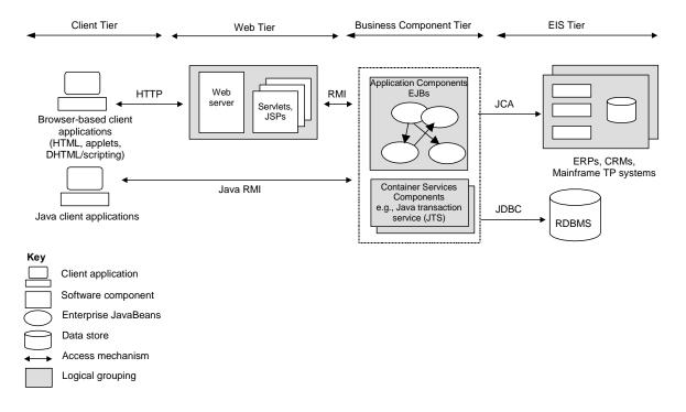
Figure 1: J2EE Multi-Tiered Application Architecture
