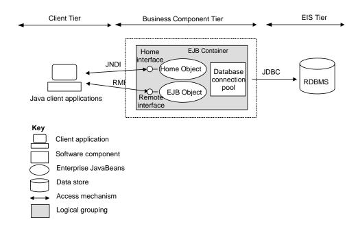
Figure 2: A Simple EJB Application Architecture
