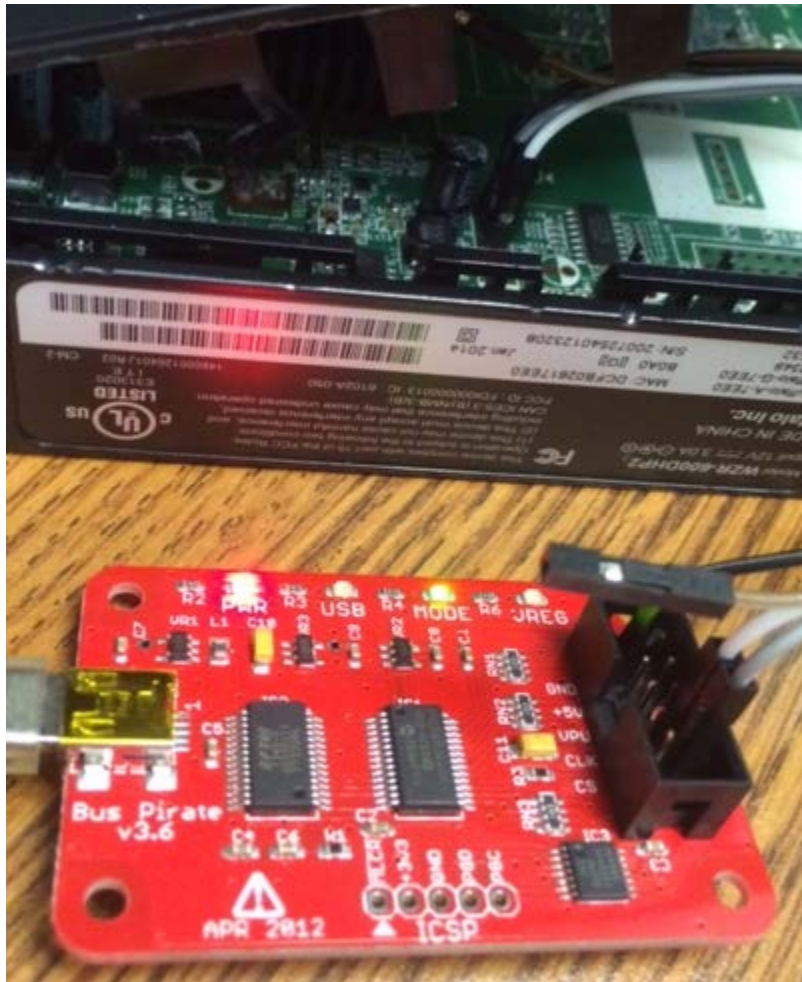
Figure 10: Buffalo UART to Bus Pirate to Terminal
