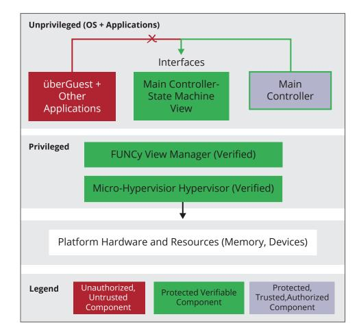
überXMHF/überSpark extended to include überobject protections for sensitive areas of the Control node and Data node.
