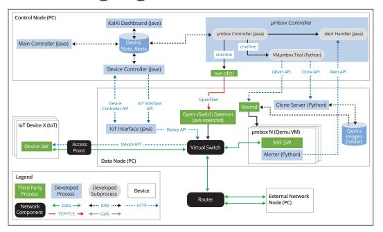
End-to-end prototype of IoT Security Platform implemented and tested with different attack scenarios. Policies and µmboxes implemented for four representative devices.
