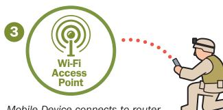
Mobile Device connects to router, validates server credentials, and authenticates with RADIUS server
