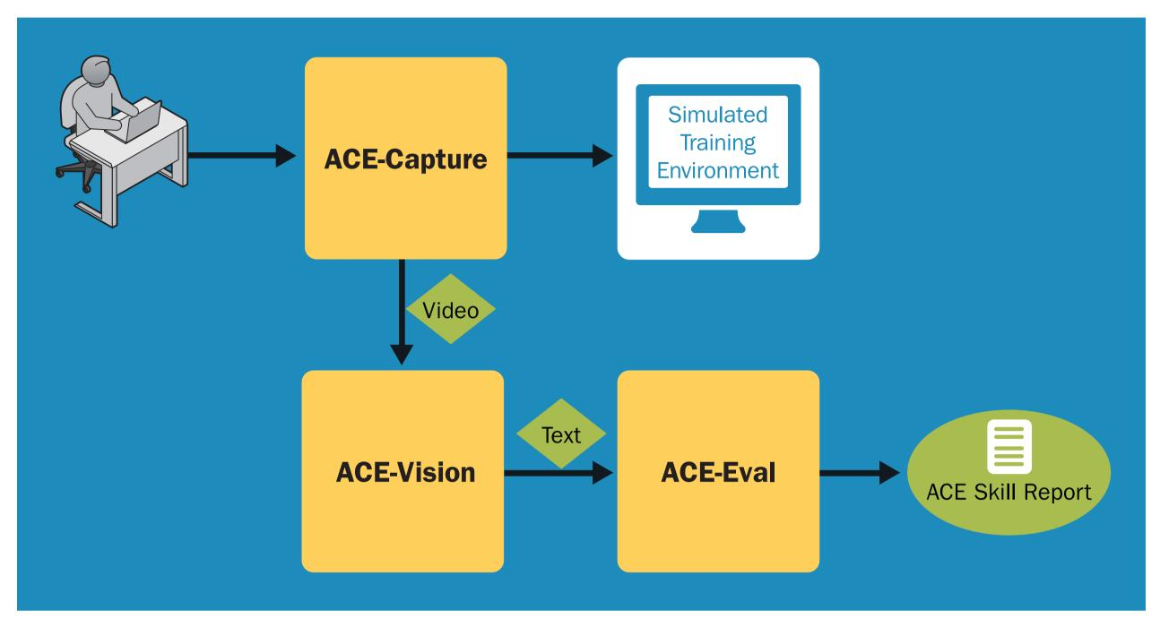
ACE Architecture Overview - User logged into Simulated Training Environment observed using Capture System. Captured video is analyzed and transcribed utilizing ACE-Vision. Vision output is processed by ACE-Eval and used to generate the ACE Skill Report.
