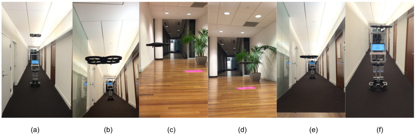
Figure 5: Coordination between CoBot and UAV to perform visual search task. (a) Drone taking off from the CoBot, (b)-(c) Drone performing forward search for target marker, (d) Drone hovering above marker after reaching it, (e) Drone performing backward search for CoBot, (f) Drone landing above CoBot.
