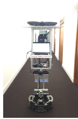
Figure 1: CoBot carrying ARDrone.
