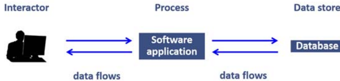
Figure 1: Data Flow Diagram for an Information System
