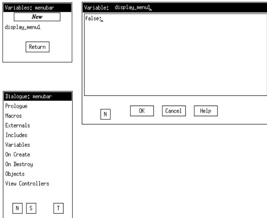
Figure 3-11 Variable Initialization for Display_menu1
